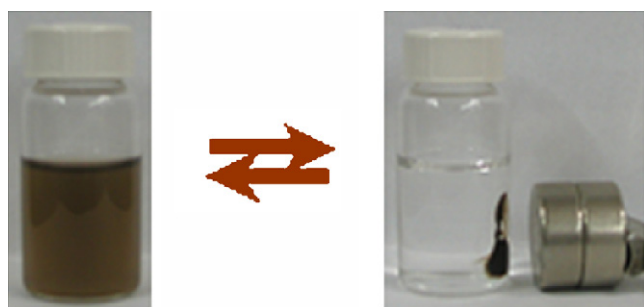
Fig. 8. Images of the magnetic nanocomposites (a) without and (b) with an external magnetic field. The aggregations were formed when an external magnetic field was applied, which dispersed rapidly when the magnetic field was removed (within few minutes).
